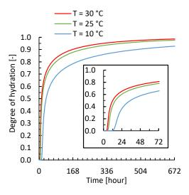
**Figure 3**: Example of the hydration curve defining the increase of the degree of hydration in time (the detail showing the first 72 hours).
