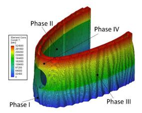
**Figure 6**: Model of the Prvok House schematically showing the construction sequence and the construction time (in seconds) of different parts of the structure.
