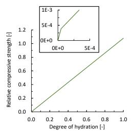
**Figure 4**: Example of a function relating the degree of hydration and relative compressive strength.
