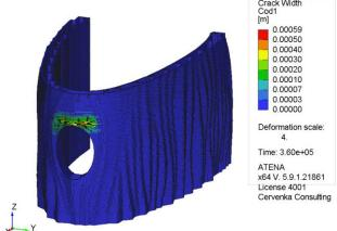
Figure 9: Distribution of the crack width over the model.
