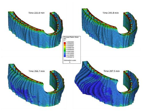
**Figure 10**: Progressive collapse of the sandwich wall for the simulation with the printing velocity increased 10x (deformation increased 5x).
