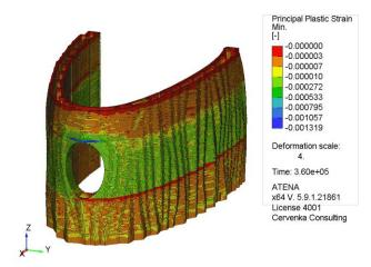
**Figure 8**: Distribution of the minimum principal plastic strains over the model.
