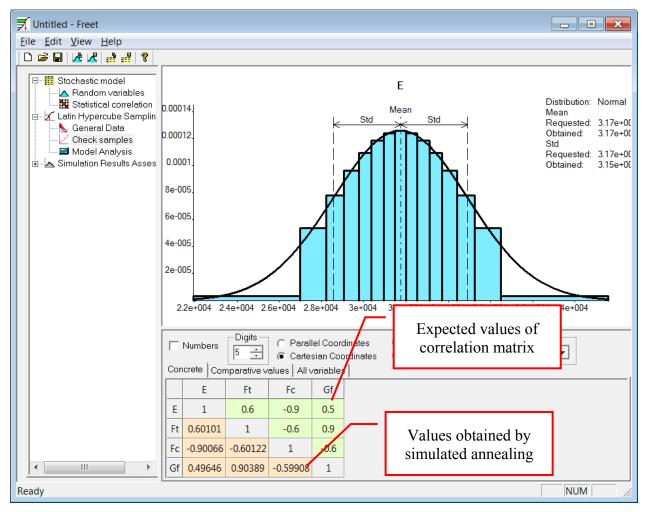
Figure 17 Freet – generated parameters
