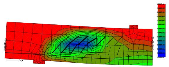
Figure 5 43. analysis step (peak): iso-areas of crack width (max. 0,36 mm)
