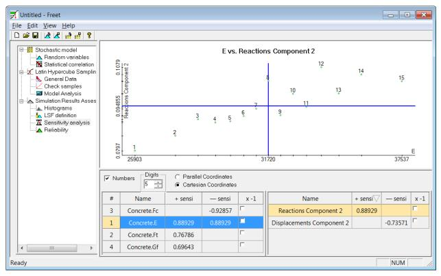
Figure 30 FREET – Sensitivity analysis of Reaction component 2 on Young's modulus E (Cartesian coordinates)
