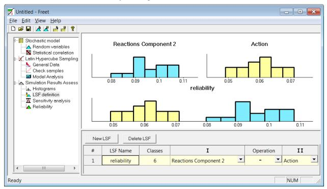
Figure 32 FREET – definition of a new limit state function
