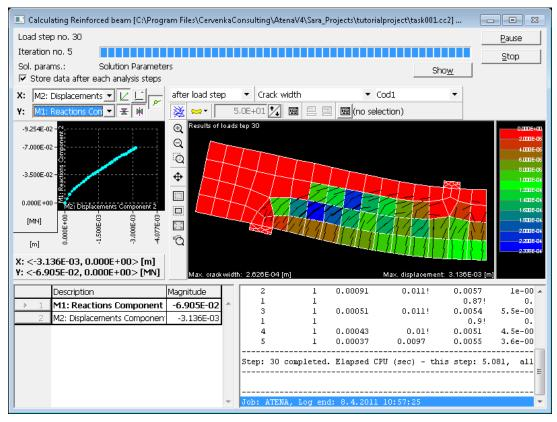
Figure 21 Analysis progress – the left window displays the LD diagram, the right shows deformed shape of the specimen (all displacements are magnified) with contours showing the crack width.
