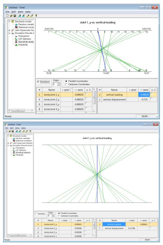
Figure 79 Negative sensitivity of maximum loading (carrying capacity of the cross section) and displacement of reinforcement. Above: simulations with 5Ø8, sensitivity is -0.989; below: 10Ø8, sensitivity is -0.996.
