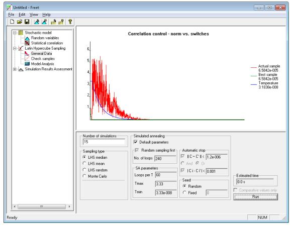
Figure 16 Freet – generation of randomized parameters
