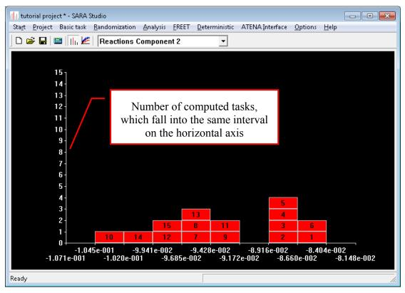
Figure 23 Finished analysis – distribution of results ordered by "Reactions Component 2"
