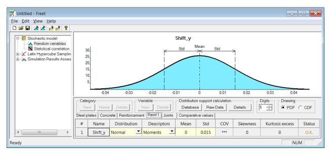
Figure 52 FReET – vertical coordinate of reinforcing bar is randomized
