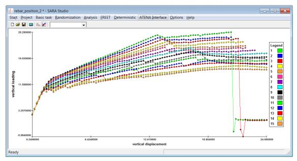
Figure 78 LD diagrams of 15 variants and additional rebars (10Ø8 in total)
