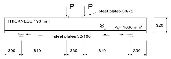
Figure 1 Geometry and loading of Leonhard's beam
