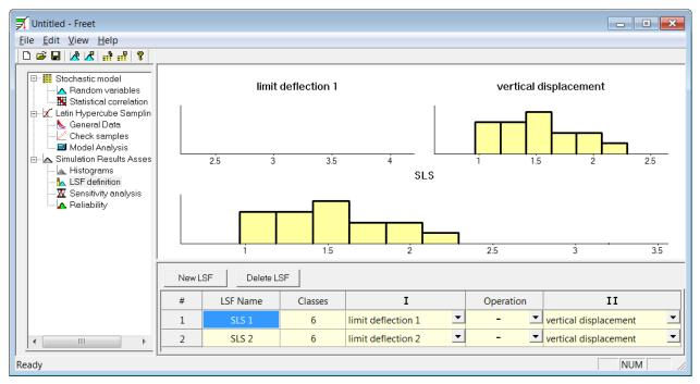
Figure 91 Definition of limit state functions.
