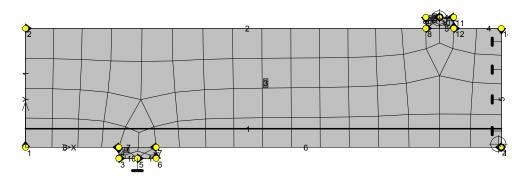
Figure 2 FE mesh, monitoring points and boundary conditions.
