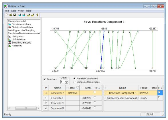
Figure 28 FREET – Sensitivity analysis (parallel coordinates)
