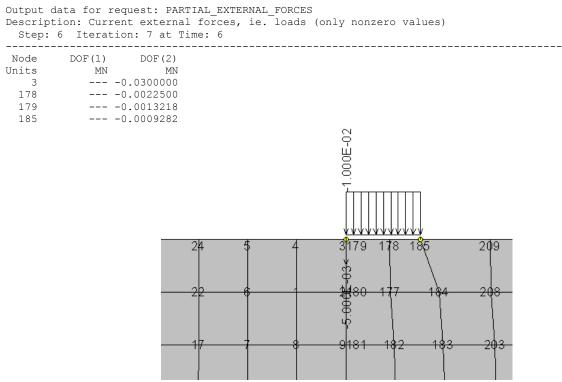
Fig. 2-12 External loading forces in double nodes located on the border of element groups.
