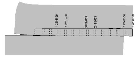
Fig. 8-17 Shear stress distribution. Load step 10, deformed object.
