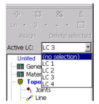
2. Selecting an active load case from a list in the menu above the access tree as shown in Fig. 4-59. The active load case can be always checked in this field.
