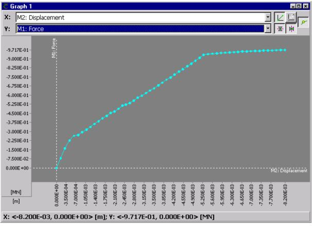
Fig. 7-2 Graph window with monitored load-displacement diagram.
