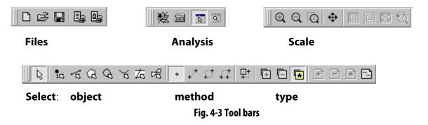
The tool bar **Select** can be used to select geometrical objects. This bar is present only in the input window (pre-processing). The selected objects are depicted by green color. The way how to select objects in the window is defined by combination of several functions as follows.
