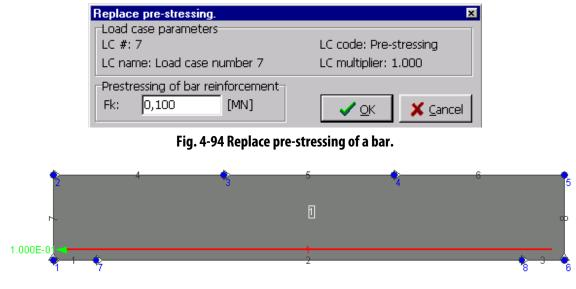
Fig. 4-95 Pre-stressing of a bar, example.
