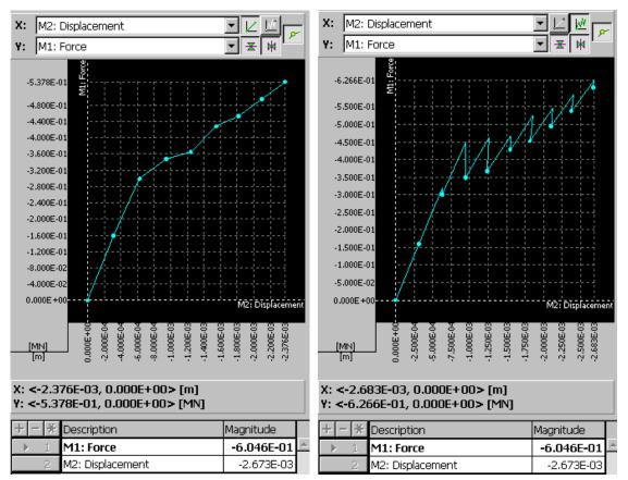
Fig. 5-7 Load-displacement diagram. Left - load steps only. Right – iterations and load steps.
