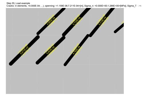
Fig. 8-12 shows a detail view of a cracked region with labels. The label contains in the first row normal stress (denoted by  $\mathbf{n}$  before the number), in the second row the crack width and in the third row the shear stress (denoted by  $\mathbf{t}$  before the number). The stresses are concrete stresses on the crack face.
