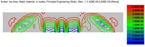
Fig. 8-21 RC beam. Maximal principal strains by contour lines.
