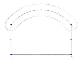
In this case 'size' is the element size along the line and 'radius' is the distance from the line where the element size given by of macroelement is resumed. An example of such refinement is shown in Fig. 4-33, where the arc line no.1 has prescribed mesh refinement by size and radius.
