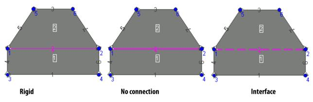
Fig. 4-54 Three types of line connection between macroelements.
