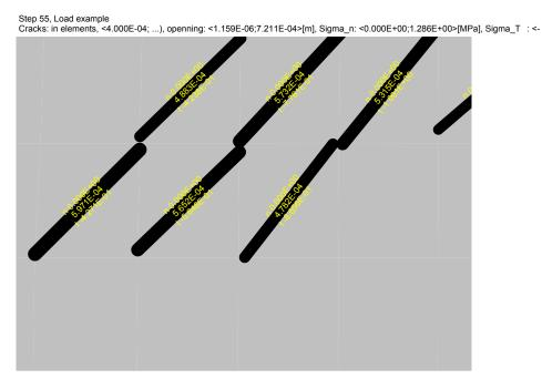
Fig. 8-12 Cracks in R.C. beam. Enlarged view of cracks with labels.
