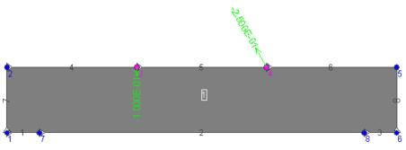
Fig. 4-64 Loading case with two forces.
