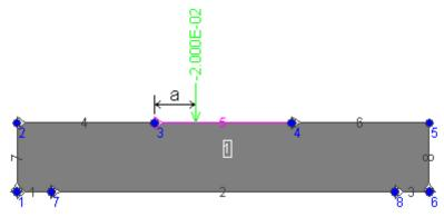
Fig. 4-68 Force within a line - example.
