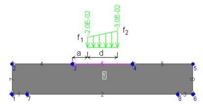
Fig. 4-71 Line load distributed on part of line – example
