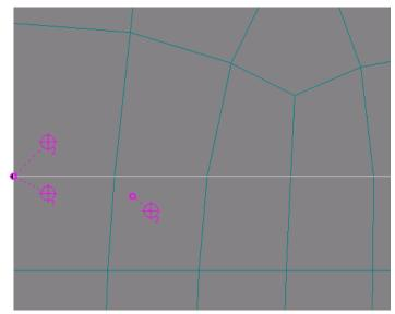
Fig. 4-104 Monitoring points – example. Relation to node and integration point.
