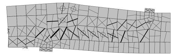
Fig. 8-11 Cracks in failing shear slab. Cracks parallel to the X-Y plane are shown as circles.
