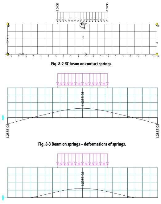
Fig. 8-4 Beam on contact springs – reaction forces in springs.
