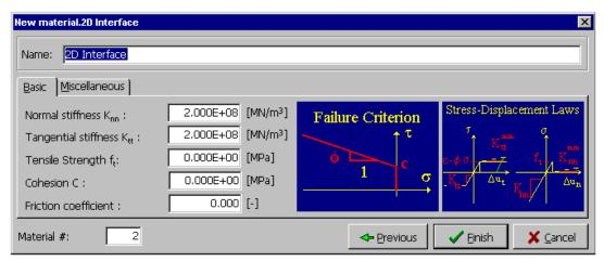
Fig. 4-13 Input of interface material.
