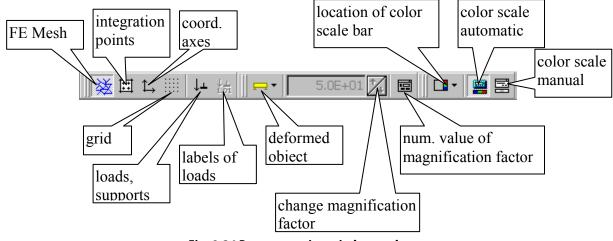
Fig. 8-24 Post-processing window tools.
