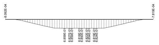
Fig. 8-6 Moment distribution. Integration in nodes (average stresses).
