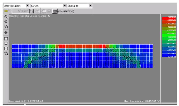
Fig. 5-10 View of cracks and stresses in undeformed mesh.
