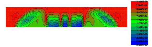
Fig. 8-20 RC beam. Maximal principal strains by contour areas.
