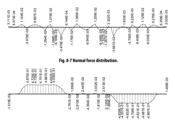
Fig. 8-8 Shear force distribution.
