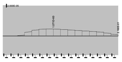
Fig. 8-16 Shear stress distribution in interface. Load step 3, undeformed object.
